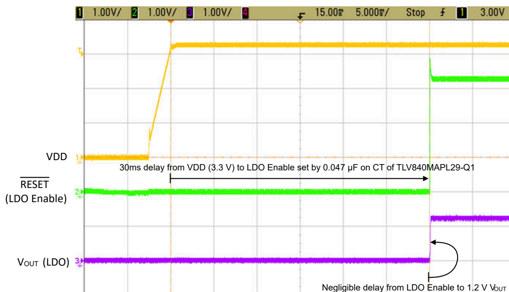
Figure 9-2. Startup Sequence Highlighting the Delay Between 3.3 V and 1.2 V Rails
