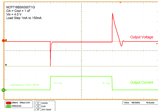
Figure 17. Load Transient Response
