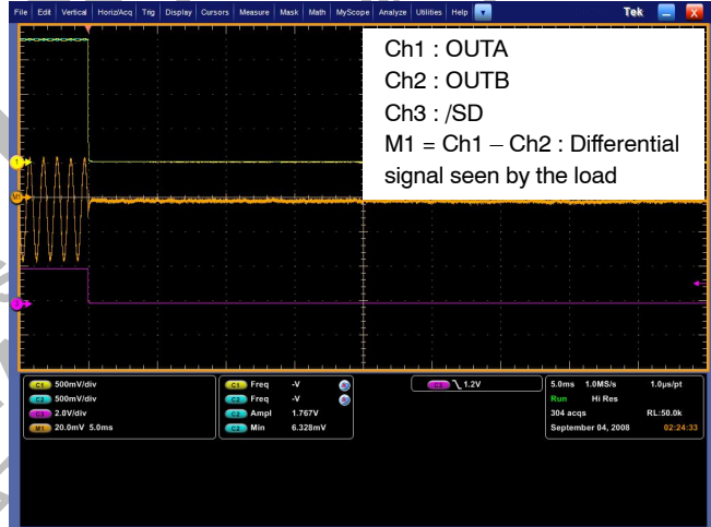
Figure 32. Zero pop noise turn off sequence with differential input audio source ( C_i = 100 \text{ nF} , R_i = 24 \text{ k}\Omega , R_f = 24 \text{ k}\Omega , C_{byp} = 1 \text{ }\mu\text{F} , R_l = 8 \text{ }\Omega , T_{on} = \text{GND} )
