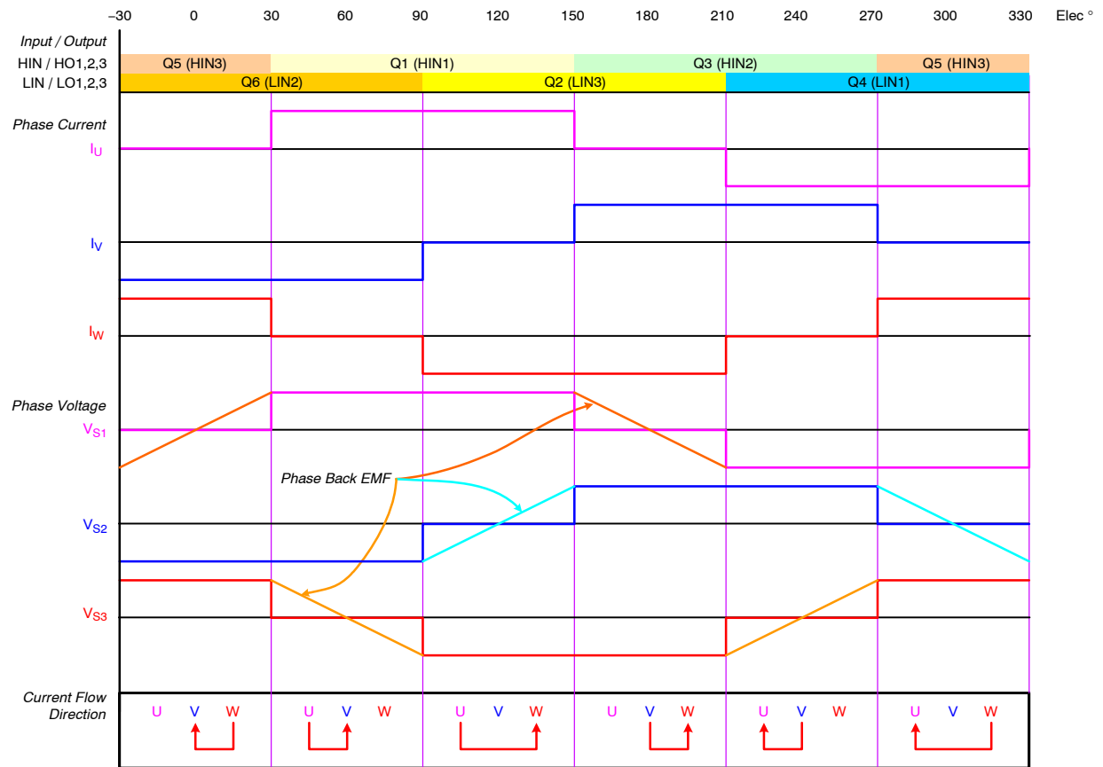
Figure 29. 120° Commutation Operation Waveforms for 3-Phase BLDC Motor Application
